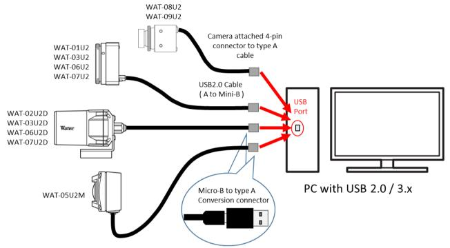
Fig.1 Watec USB Camera - PC Connection Example
