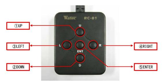
Figure 1. RC-01 (remote controller)
